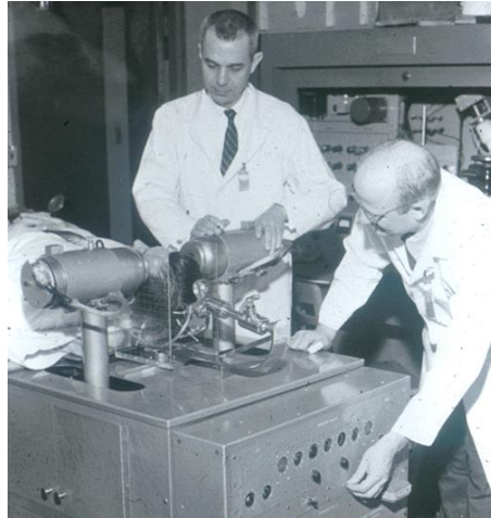
Fig 1: First Clinical Positron Imaging Device
